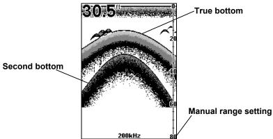
Example of a second bottom signal. Unit is in 30 feet of water, with range set at 80 feet and sensitivity set to 87 percent
